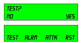
To exit the 'TEST' mode press and hold the key assigned to RST (reset) for about 3 seconds.
