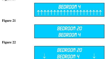
From the speaker within the NET243 an audible tone can be heard relative to the alarm condition of line 1 on the LCD. If there is any confusion as to what the sound is indicating, press the **ADJUST** button momentarily to reveal the "**statistics window**" (Identification number, alarm condition and the time at which the call was initiated).
